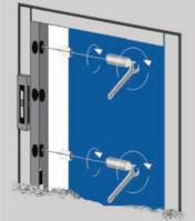
There are 12 adjusters supplied per door (additional can be purchased if required) and 24 positions (12 on each side) into which adjusters can be secured.
